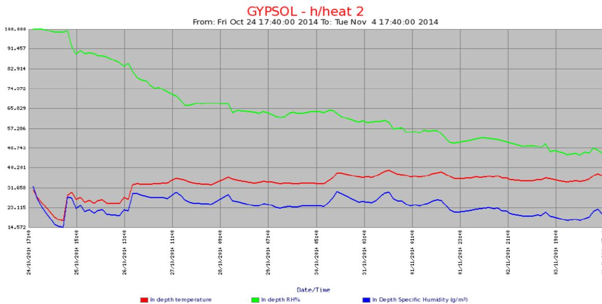
Figure 1 - Relative Humidity (in green) steadily drops after commissioning of underfloor heating.
