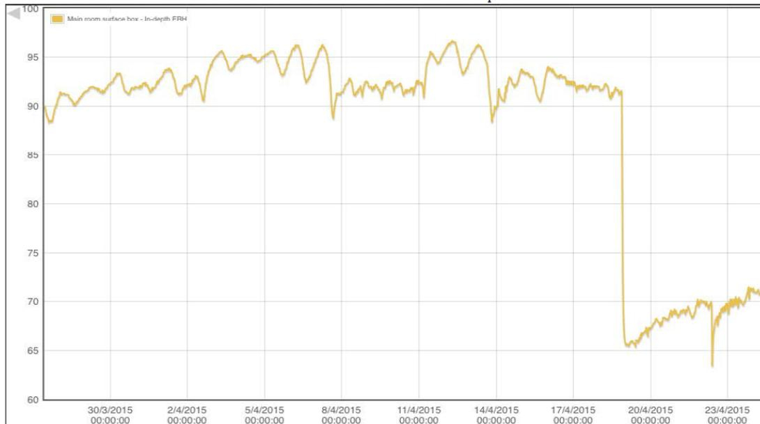
Figure 3 - Using the reference method of surface box RH the 50mm Gypsol screed dries in 27 days.
