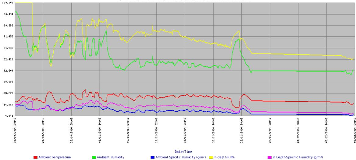
Figure 2 - Relative humidity (in green) in standard conditions reaches <75% within 27 days from installation of a 40 mm Gypsol screed.
